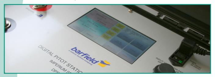
The DPS1000 is Barfield's latest fully automated, user-friendly RVSM compliant air data test set. Replacing the DPS350, the DPS1000 performs altimeter and static systems tests and inspections. Critical components used in the DPS1000 have a well established history of proven flight line accuracy including pumps, valves and static/altitude transducers.
